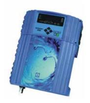
**Testomat 2000** for monitoring of the max. allowed residual hardness after Evoqua water softening systems by periodic chemical analysis with threshold indicators (tritration and colorimetric determination).
