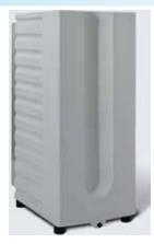
Storage tanks with conical bottom for pure water are constructed from polyethylene to minimise the release of organics. Vent filters prevent the ingress of airbourne impurities. Further accessories see below. Level control with pressure sensor (4 - 20 mA).
