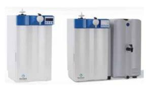
The LaboStar® 10 RO DI system has a small foot print and produces pure water with a quality of up to 10 M $\Omega$ -cm. The versatile system includes a 7 L storage tank with the option of adding a 30 I or 60 I tank. The pure water is collected in a tank and transferred by a built-in circulation pump. Typical applications are IC, Pathology, Buffer preparation, general chemistry, feed for laboratory ultrapure water systems etc.
