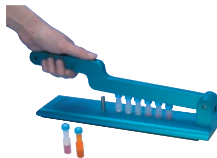
Fig 4: The multicompressor of the Mini-UniPrep polypropylene version holds 6 vials.
