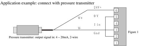
Use with 2-wire pressure transmitter/ sensor. The instrument can supply DC 24V auxiliary power, and the sensor output is 4 ~ 20mA. Software select input signal mA. Please refer to above figure 1.
