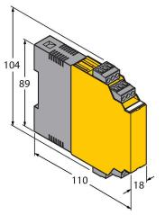
Isolating switching amplifier, 2-channel; 2 relay outputs; input NAMUR signal; selectable ON/OFF mode for wirebreak and short-circuit monitoring; adjustable output mode (NO / NC mode); removable terminal blocks; width 18 mm; universal power supply unit
