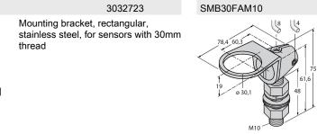
Mounting bracket, stainless steel, for M10 x 1.5 thread, thread length 30 mm
