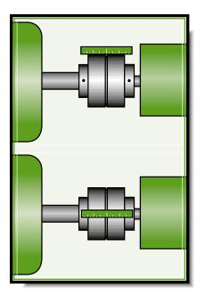
Perfect alignment of equipment shafts, in most cases, is impractical to obtain or maintain, and misaligned equipment produces excess stress on bearings and coupling. Magnaloy's insert design will accept misalignment strain and, when excessive, will cause insert wear as a visual and audible indication of misalignment problems. However, Magnaloy's inserts are inexpensive and easily replaced; under normal conditions the insert seldom requires replacement.
