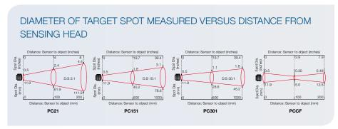
All PyroCouple sensors are fitted with precision Germanium lenses for accurate optics. Model PC21 has 2:1 optics making it suitable for most applications where the sensor can be mounted close to the target. Model PC151 is designed for small or distant targets and has an optical resolution of 15:1. Model PC301 is designed for very small or distant targets and has an optical resolution of 30:1. Model PCCF is designed for targets as small as ø5mm at a distance of 100mm from the sensor.
