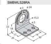
Mounting bracket, angled, metal, for WLS28 work lights, 5 mm drill holes, screw set included
