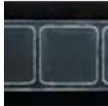
Only the edges are extracted. The position detection of stickers can be precisely carried out.
