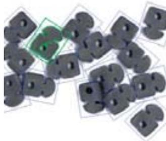
ShapeTrax II detects the position of multiple parts, even if they are overlapped.
