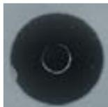
The chip on the edge appears bright and is clearly recognised.
