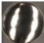
The print is not detected because of irregular reflection from the curved can bottom.
